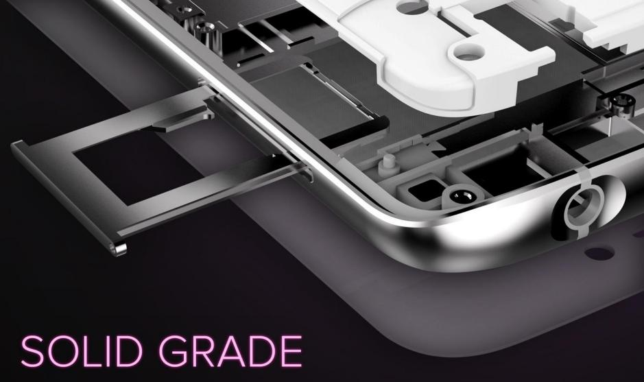
BLU set out to engineer a remarkable device that combines different elements including metal and glass. To fuse the two materials together, a combination of nano-molding, laser welding and CNC techniques on the zinc alloy metal form a reliable and aesthetically sound infrastructure. The back cover is constructed of glass which gives the device a smooth and sexy look. The Studio One is a metamorphosis of technology and tasteful design that brings premium quality to the consumer.
